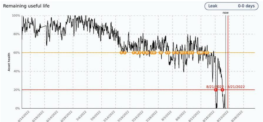
IMAGE 4: Later progression of a reciprocating compressor valve fault. Times when warning alerts are triggered are depicted with yellow dots. Critical alerts are depicted with red dots.
