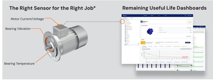
\*Novity TruPrognostics can monitor electric motors using data from several combinations of the above sensors.
